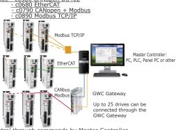
Drive control through commands by Master Controller. Suitable for multi axes systems (up to 127 drives). Built in powerfull Motion Module functionality assures perfect synchronization among axes and reduces Master Controller workload
